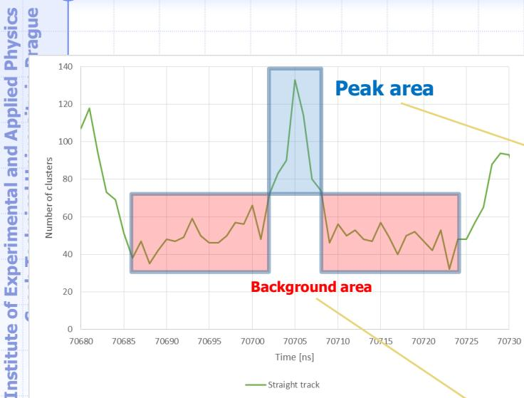
In the peak area in addition to the events also seen in the background area, highly aligned tracks (possibly MIPs from the interaction point are seen).
