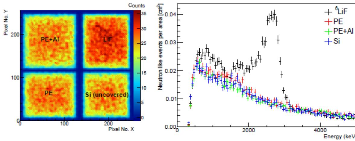
$$\Phi_{n,i} = \frac{N_i/A_i - N_{Si}/A_{Si}}{\epsilon_i N_{\text{frames}} t_{\text{acq.}}}$$
